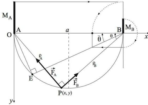
**Figure 7.** Sketch of the half circular path bicentral motion, and its equilibrium point.
