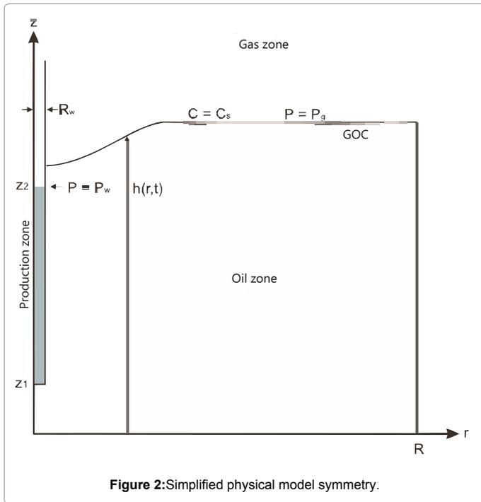
Figure 2: Simplified physical model symmetry.
