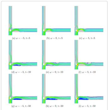
Figure 3: Effect of cylinder rotation angle on the streamlines for fixed value of Re=300.
