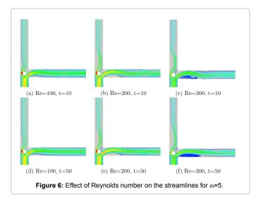
The length of the recirculation zone is seen to increase in a nonlinear fashion with an increase in Reynolds number for a particular angle of rotation. The recirculation length is also seen to increase with decreasing angle of rotation for a fixed Reynolds number. Thus, the dimensional considerations suggest that the recirculation length is a function of Reynolds number and angle of rotation.
