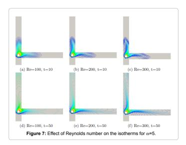
the installation of the rotating cylindrical obstacle. The result shows the effect of rotation on the local Nusselt number distribution is more pronounced at low Reynolds number.
