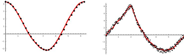
Figure 3. Comparison between the noisy Cauchy data on  $\Gamma$  and the computed data on the inverse problem (first simulation). On the left– first coordinate of the solution, on the right– second coordinate of the traction vector. Dots– data from the direct problem, thick red line– inverse problem. Noise level: 8 %.
