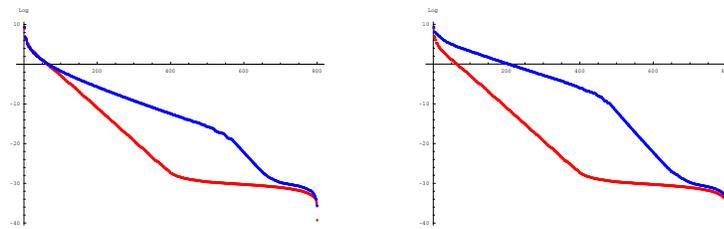
Figure 10. Eigenvalues of the system arising from the discretization of the problems: Left- Inclusion reconstruction (homogeneous Dirichlet condition on  $\gamma$ ); Right- cavity reconstruction (homogeneous Neumann condition on  $\gamma$ ). Blue (top) curve- direct problem using MFS; Red (bottom) curve- inverse problem using the Kirsch Kress method.
