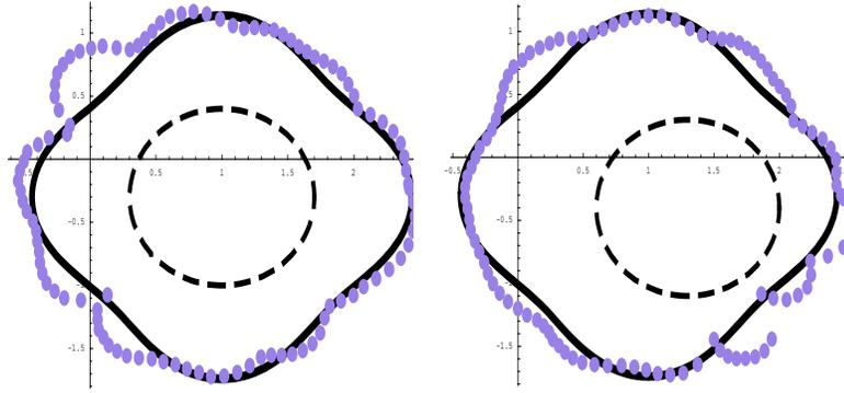
Figure 6. Reconstruction of the shape with internal circle (dashed line) centered with the inclusion (left) and on  $(1.3, -0.4)$  (right). Noise level: 8 % .
