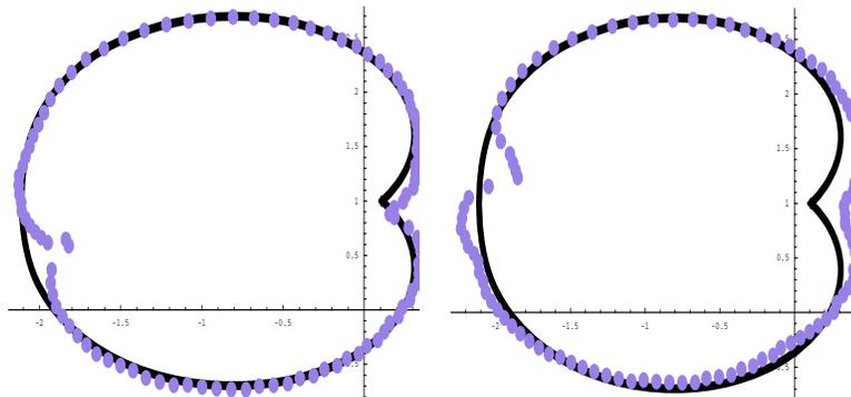
Figure 5. Reconstruction of the shape with 3 % (left) and 8 % (right) of noise. Full line- Shape of the inclusion; Dotted line- Reconstructed curve.
