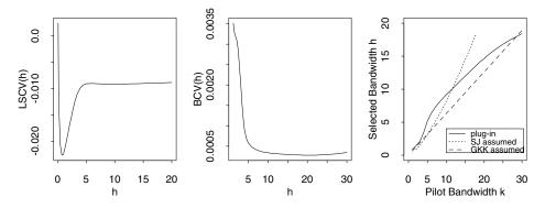
$\label{eq:Fig. 10.} \textit{Informative bandwidth selection: The LSCV criterion (left); BCV (middle) and plug-in (right).}$
