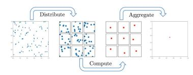
Fig 1: Distributed estimation protocol where data is randomly distributed across nodes to obtain "local" estimates that are aggregated to compute a "global" estimate.
