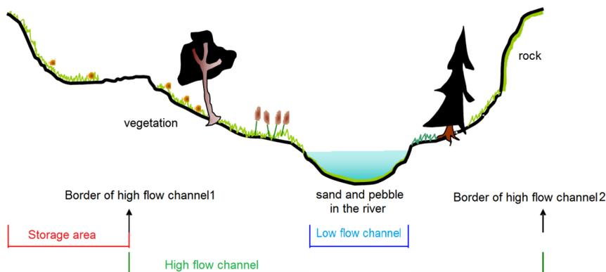
FIG 5. Representation of a river cross section, showing the main channel (low flow channel) and the flood plain (high flow channel). Source: [28].
