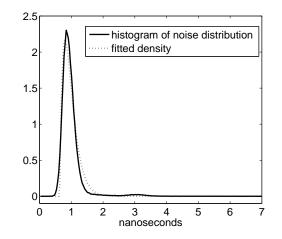
FIG 1. Normalized histogram based on a sample of the noise distribution (solid line) and the fitted density (dashed line) having the form of (20) with  $\hat{\alpha} = 0.961$ ,  $\hat{\beta} = 0.941$ ,  $\hat{\nu} = 5.74$ ,  $\hat{\tau} = 5.89$ .
