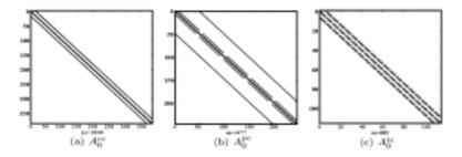
Fig. 3. Sparsity of the coefficient matrices  $A_0^{cc}$ ,  $A_0^{pc}$ , and  $A_0^{ic}$ . (a)  $A_0^{cc}$  with matrix size 384, (b)  $A_0^{pc}$  with matrix size 245, and (c)  $A_0^{ic}$  with matrix size 114.
