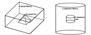
Fig. 1. Structure schema of a pyramidal and a cylindrical quantum dot. Each of the quantum dots is embedded in a hetero-structure matrix.
