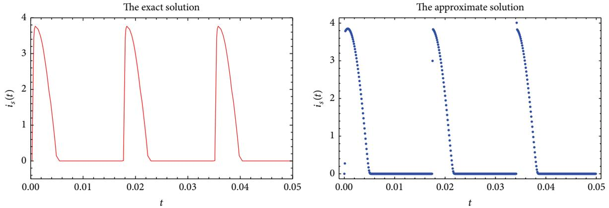
FIGURE 2: The exact and approximate solutions for the current of the diode circuit.
