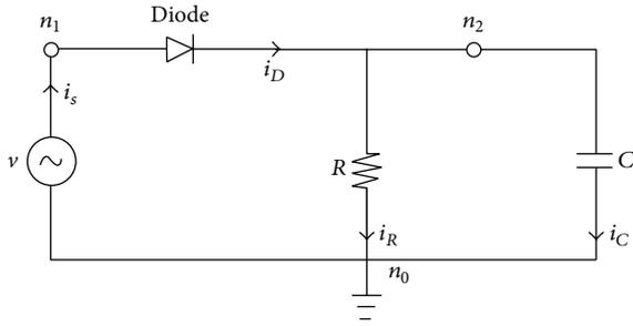
FIGURE 1: Rectifier circuit.
