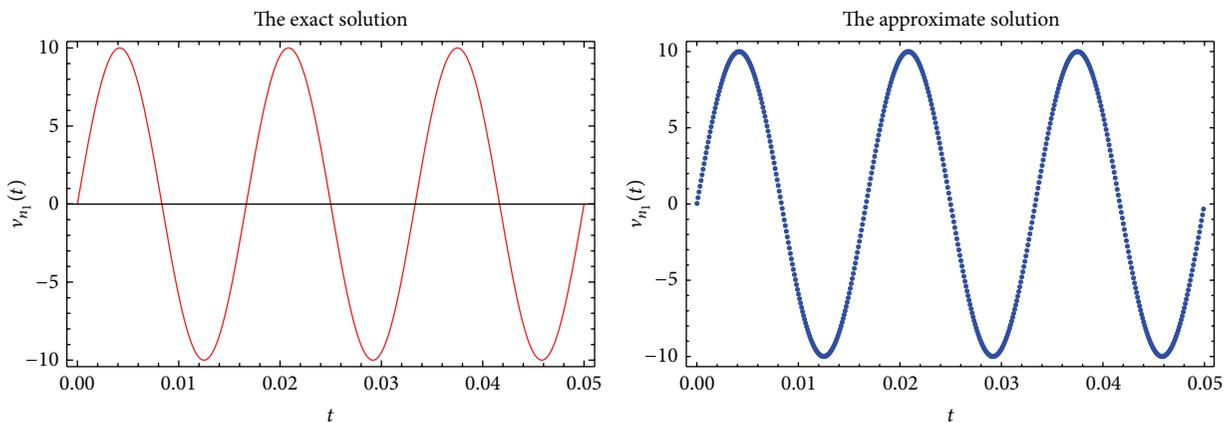
FIGURE 4: The exact and approximate solutions of the voltage ( $v_{n_1}(t)$ ) of the diode circuit.
