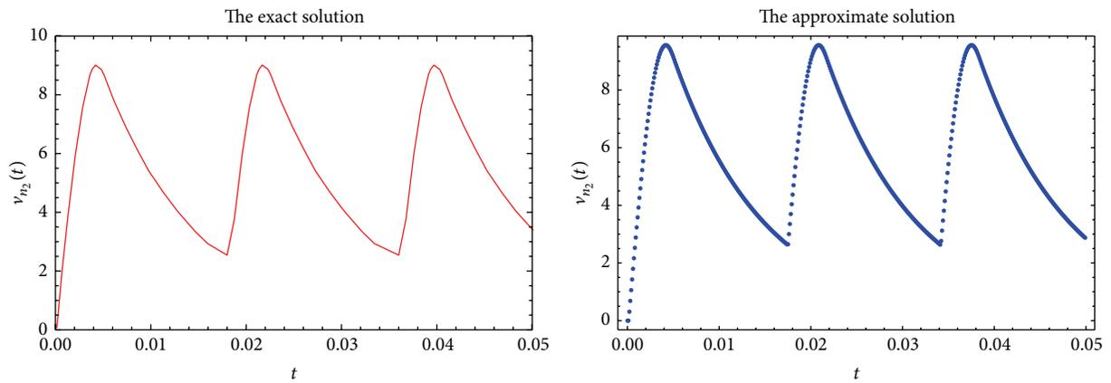
FIGURE 3: The exact and numerical solutions for the voltage ( $v_{n_2}(t)$ ) of the diode circuit.
