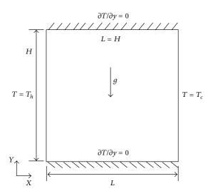
FIGURE 1: Schematic of analyzed configuration.
