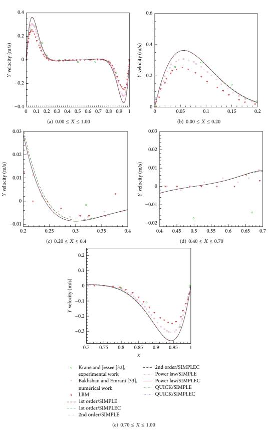
FIGURE 3: Vertical velocity profile at midheight.
