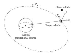
FIGURE 1: Relative Cartesian coordinate system for spacecraft rendezvous.
