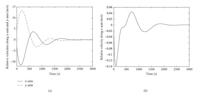
FIGURE 3: Relative velocities between two spacecrafts along each axis.
