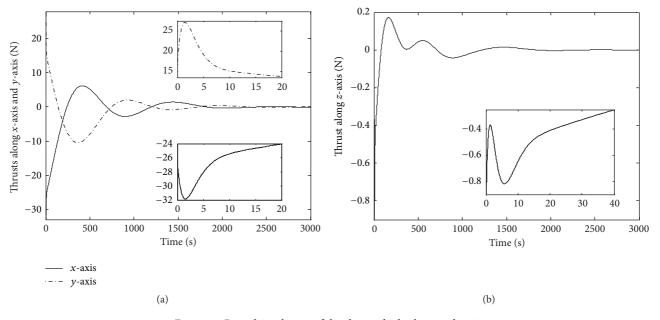
FIGURE 4: Propulsive thrusts of the chase vehicle along each axis.
