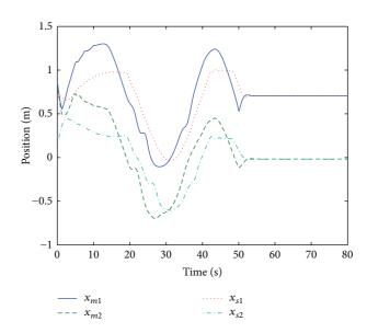
FIGURE 6: The positions of the master and the slave in task space with the known gravity term.
