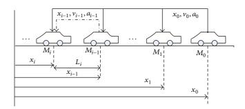
FIGURE 1: Spacing errors in a platoon.
