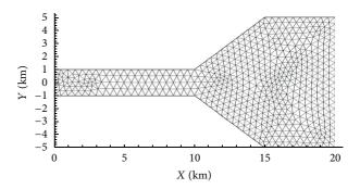
FIGURE 2: Mesh setup of generalized estuary.
