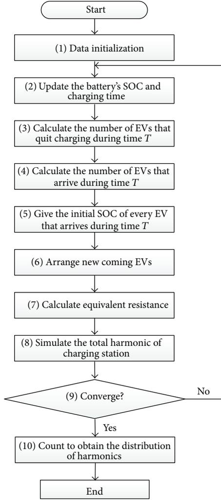
FIGURE 6: Calculating the EV charging station's harmonic distribution.
