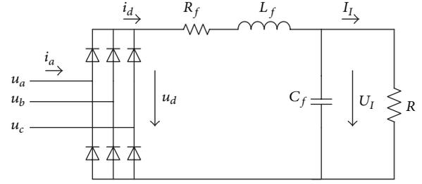
FIGURE 1: The structure diagram of equivalent simplified mode for EV charger [20].
