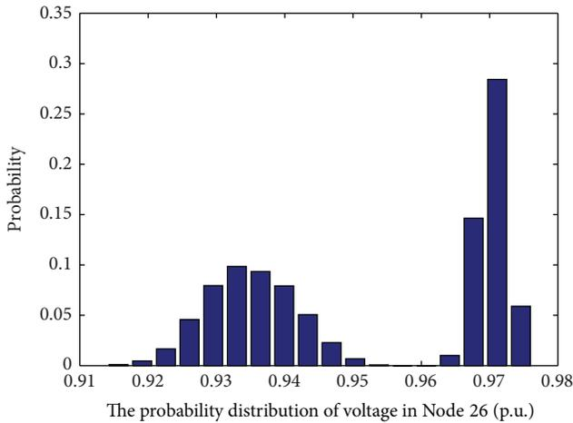
FIGURE 11: The probability distribution of voltage in node 26.
