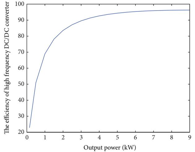
FIGURE 2: The relationship between efficiency and output power.
