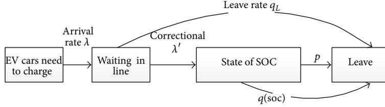
FIGURE 5: The correctional diagram of EVs' charging process.
