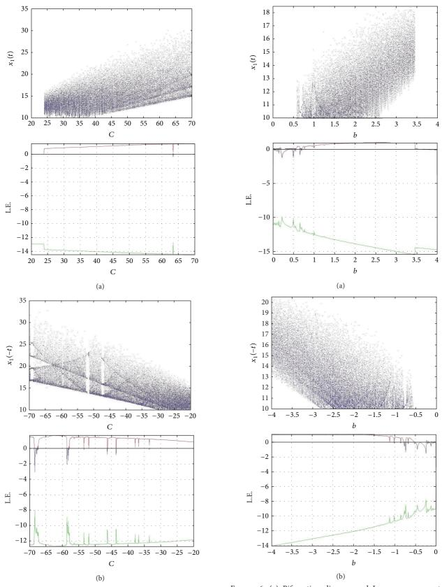
FIGURE 5: (a) Bifurcation diagram and Lyapunov exponents of chaotic classical Lorentz system with b=8/3 and a=10. (b) Bifurcation diagram and Lyapunov exponents of chaotic timereversed Lorentz system with b=-8/3 and a=-10. The tables given previously show the different dynamic characters between classical and time-reversed Lorentz.
