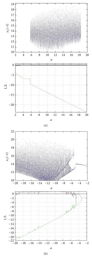
FIGURE 7: (a) Bifurcation diagram and Lyapunov exponents of chaotic classical Lorentz system with b=8/3 and c=28. (b) Bifurcation diagram and Lyapunov exponents of chaotic timereversed Lorentz system with b=-8/3 and c=-28. The tables given previously show the different dynamic characters between classical and time-reversed Lorentz systems with different ranges of parameter a.
