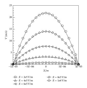
FIGURE 6: The velocity magnitude profiles under different applied electric field.
