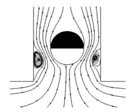
FIGURE 5: The flow diagram around the Janus cylinder when E = 2e5 V/m.
