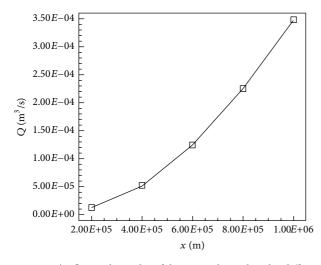
FIGURE 7: The flux at the outlet of the microchannel under different applied electric field.
