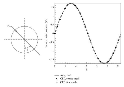
FIGURE 3: Schematic diagrams of induced zeta potential distribution on the polarizable particle's surface.  $E_0 = 42.76 \text{ KV/m}, r = 20 \, \mu \text{m}.$
