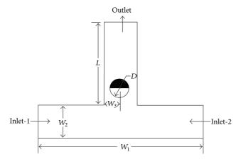
FIGURE 1: Schematic diagram of the T-shaped microchannel with Janus cylinder.
