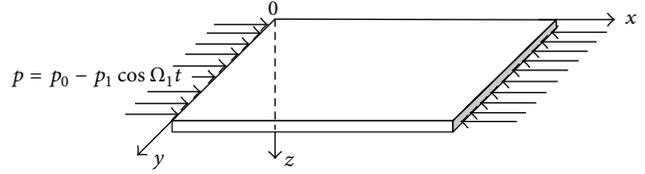
FIGURE 1: The model of a rectangular thin plate subjected to parametrical excitation.
