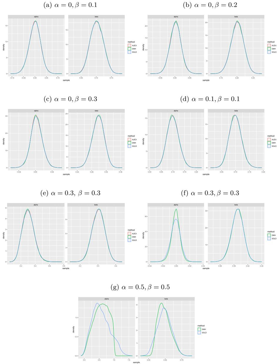
Figure 1: Density plots of posterior samples generated by AUEx, DMH and SGLD under different settings of  $(\alpha, \beta)$  for the spatial autologistic model.
